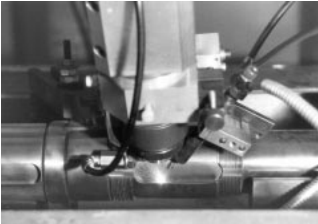
Fig. 10 Precision laser beam cladding of oversized groove in a finished shaft (base material 0.45% carbon steel, cladding Stellite material)
