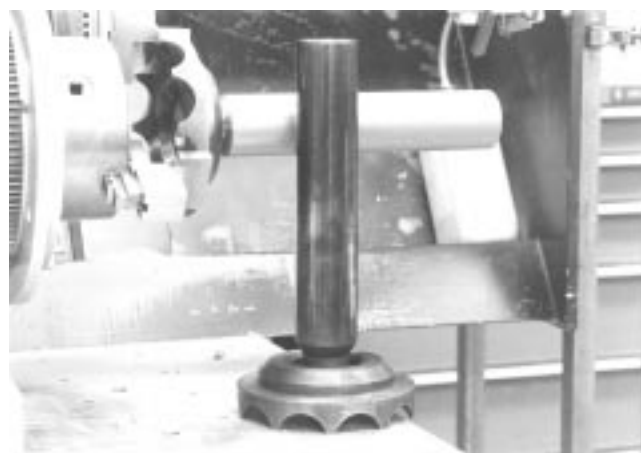
Fig. 9 Repaired and worn (standing) plungers (base material 31CrMo12, cladding material NiCrBSi)
